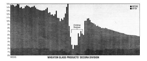
An Analysis of Wheaton Glass Products' Decora Division's rejected items shows a reduction from 14% to less than 2% after corrosion and settling problems in the glass-etching process were solved.
