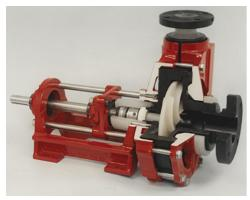
Cut-away of Vanton Chem-Gard® polypropylene pump with PVDF impeller and PVDF thick sectioned shaft sleeve. These horizontal centrifugal pumps helped solve the severe corrosion/abrasion problem created by the pumping of an etching solution of hydrofluoric acid and a proprietary powder compound. Both metal and FRP pumps previously specified for this service resulted in repeated failures and costly maintenance.
