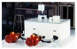
Polypropylene tank, 32" x 20" x 14" high equipped with Vanton close coupled, self-priming sealless, duplex flexible liner pumps which move wastes via overhead line from center island sinks to outside wall, where they combine with other lab wastes. Pump bodies are polypropylene; flexible liners are made of Dupont Nordel.
